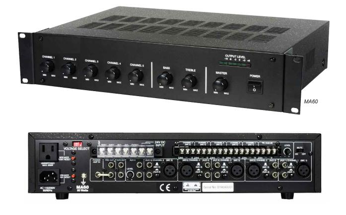
Mixer/Amplifier models MA60 (60W), MA125 (125W), and MA250 (250W) have identical features except for the maximum power output (60W, 125W, 250W) and weight. The units are powered via switchable 115 or 230 VAC @ 50/60Hz or 24VDC. Includes five channel volume controls, treble and bass controls, master volume control, main power switch, and LED display bank for output level.
